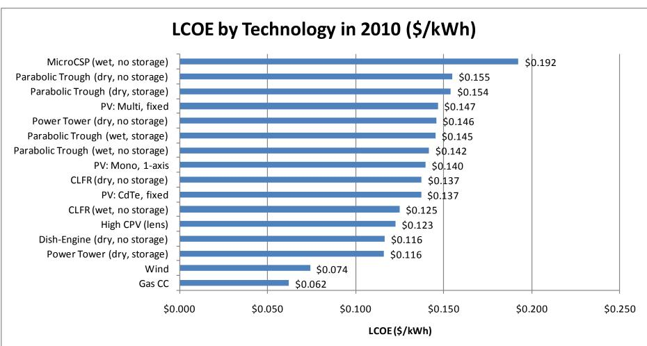
LCOE for a 250 MW plant in the US Southwest (DNI 2,500 kWh/m^2/yr). Includes 30% Treasury Grant and Accelerated Depreciation. Source: GTM Research. Prepared by Brett Prior (prior@gtmresearch.com)
